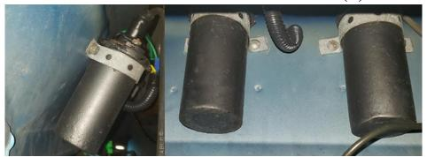
The flame coil(s) included in the kit use the Torch Control Box to provide spark to the tailpipes. These can be mounted outside and under the car's rear bumper for optimal use.
