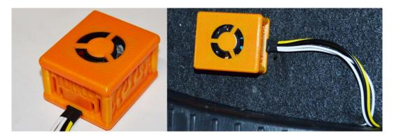
The Torch Control Box is the brains of the setup. It allows the kit to provide a hot and steady spark to the spark plugs in the tailpipes.
