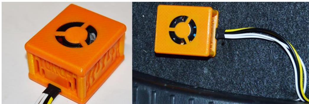
The Torch Control Box is the brains of the setup. It allows the kit to provide a hot and steady spark to the spark plugs in the tailpipes.
